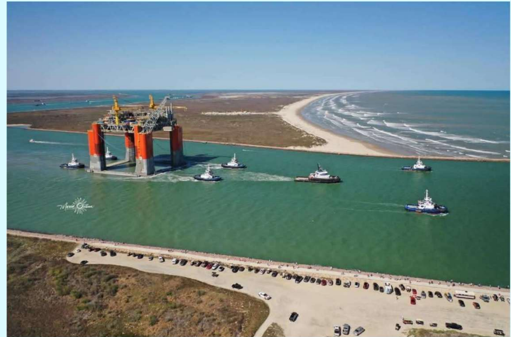
The FPS sail away to its final location above the Shenandoah field
